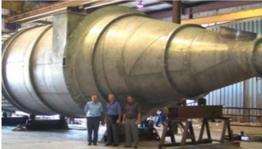
Mikropul Cyclone filter Max 40 bar, any steel/alloy type etc. Above 25000 is special design.
