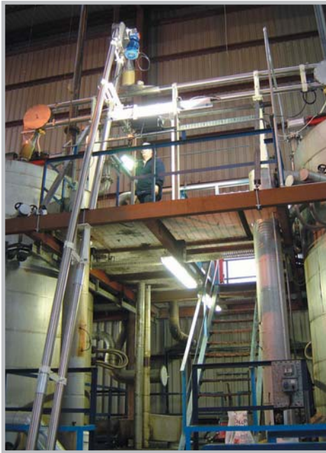
Aero mechanical conveyors are ideal for difficult products such as titanium oxide and other products which have tendency to smear or are cohesive.
