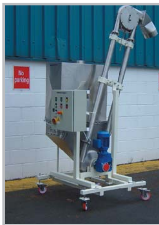
Mobile aero mechanical conveyors are used extensively both in and out of the factory environment.
