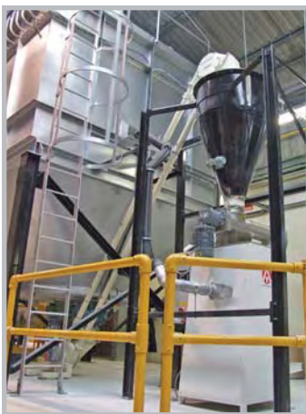
Aero mechanical conveyor elevating chemicals. Discharge heights can be specified for individual requirements.
