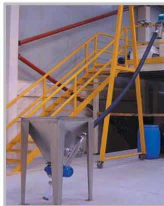
Our range of 'Rhinoveyor' Flexible Screw Conveyors are for very abrasive applications such as sand, cement, minerals and aggregates.
