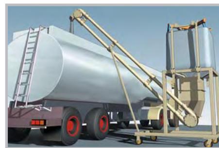
Aero mechanical conveyor mounted on a mobile frame loading road tankers.
